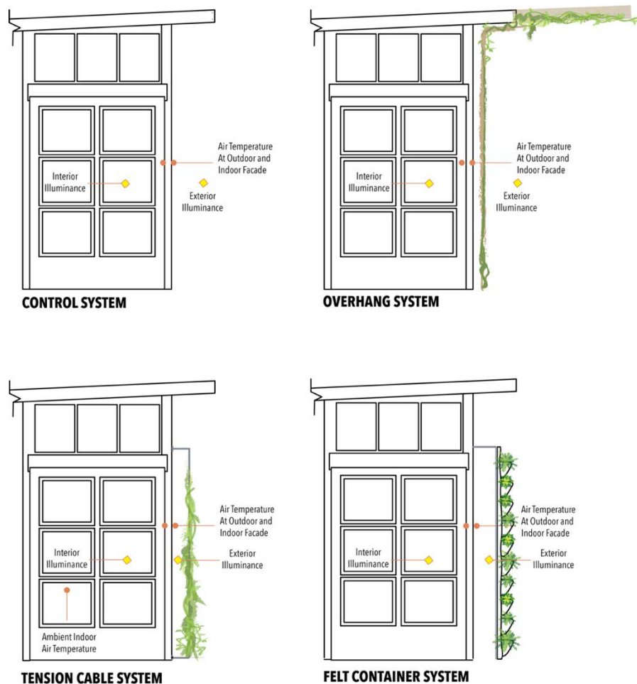
Figure 68. Reading Locations for Field Test Data Recording
