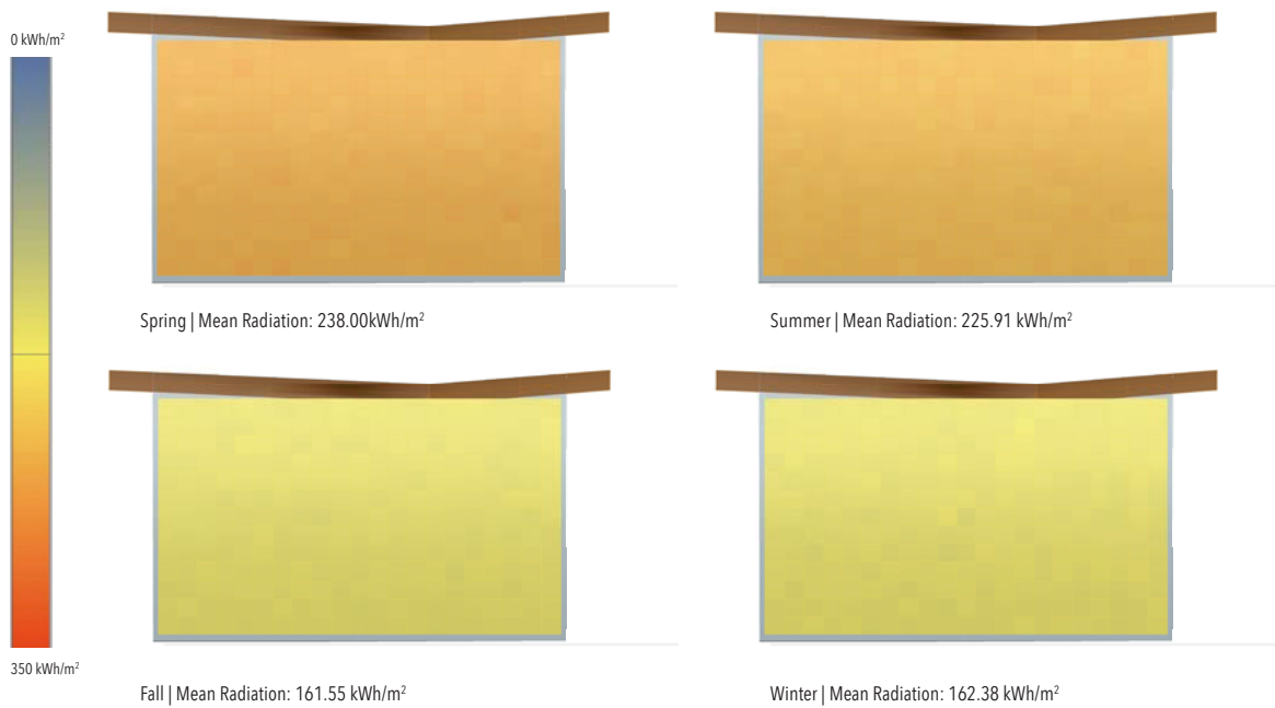
Figure 42. Seasonal Radiation Map of the East Façade of the E. 34 Greenhouse (Diva-for-Rhino)
