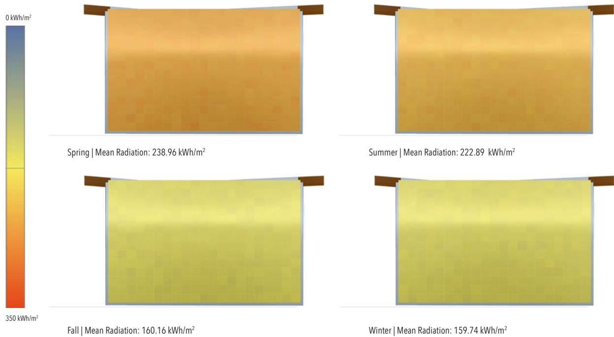
Figure 43. Seasonal Radiation Map of the West Façade of the E. 34 Greenhouse (Diva-for-Rhino)
